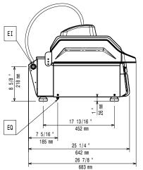
Electrical inlet (power) Electrical Outlet EO
